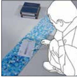
The colour blending consists of a series of mixed sheets (modules) with colours which fade into each other. Each module has eight sheets - numbered from 1 to 8 - from the lightest to the darkest colour.
